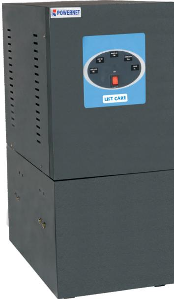
**Powernet ARD (Lift Care)** is an external emergency power supply for original lift controller. These specially designed ARD Inverter sense the Power failure / single phasing & feed the power to lift controller, to drives the lift car to the nearest floor or ground floor. Lift controller will open the door and allows the passenger to exit. This smart Rescue Device is the safest evacuation device as it has no interface with safety circuit of elevator
